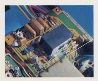
FM IF Stages. The IF section of the KR-7400 is equipped with permanently aligned solid state filters for high selectivity (80 dB), superb capture ratio (1.3 dB) and superior AM suppression (70 dB). Spurious signal rejection is more than 100 dB.
