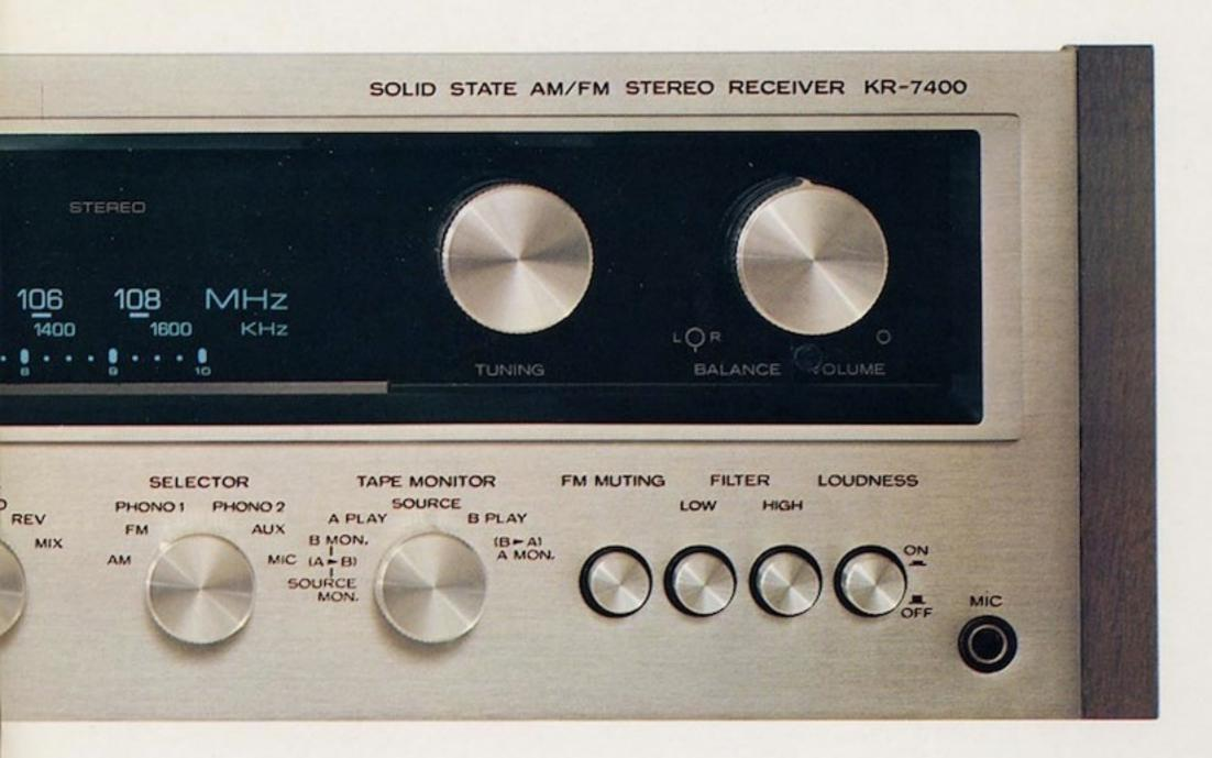
Linear FM Dial Scale. A linearfrequency variable capacitor permits the FM dial scale to be equally calibrated over its full span from 88 to 108 MHz. Combined with large signal and tuning meters, it adds up to effortless and more accurate tuning.
